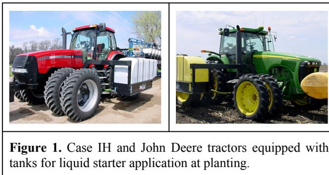
**Figure 1.** Case IH and John Deere tractors equipped with tanks for liquid starter application at planting.
